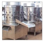
Feather Plucker for 5 to 15 birds, 24" to 30" diameter, feather discharge hopper and bird discharge hopper
