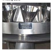
Rotating cone stand with revolving cones for Killing & Bleeding - 8 to 24 cones, Single tier and Two tier, blood collecting trough
