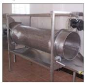
Removes excess water from the dressed bird, water collection tray
