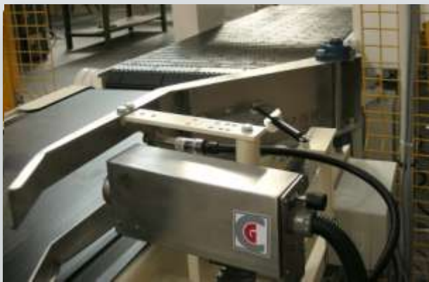
Ink-jet printer for printing on the sides of the filled bag.
