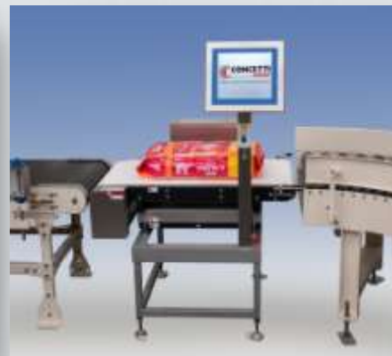
Check weigher for the filled bags.
