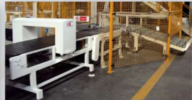
Metal detector and roller system for the bag rejection.
