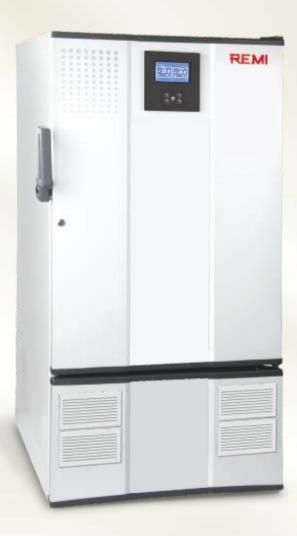
The REMI Humidity Chambers are designed for testing of electronic, electrical components, corrosion studies on mechanical parts, shelf life studies on paints, varnishes and cement at respective manufacturing facilities. These chambers control precise temperature and humidity.
