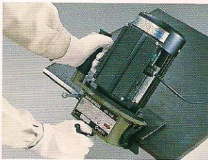
Chamfering steel plates
