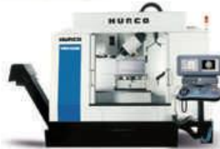
VMX42SR (5-Axis) Travel 1067 x 610 x 610 mm C=360°, B= -91/+91° Spindle 12000 rpm Total Stations 40
