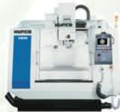
VM20 Travel 1016 x 508 x 508 mm Spindle 10000 rpm Total Stations 20
