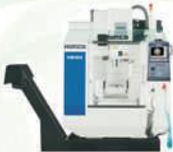
VM10U (5-Axis) Travel 533 x 406 x 483 mm C=360°, A= -30/+110° Spindle 10000 rpm Total Stations 20
