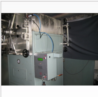
Fully Automatic Horizontal Rectangular Autoclaves with Inter Locking Double Doors
