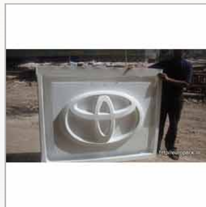
Vacuum Forming Thick Sheets
